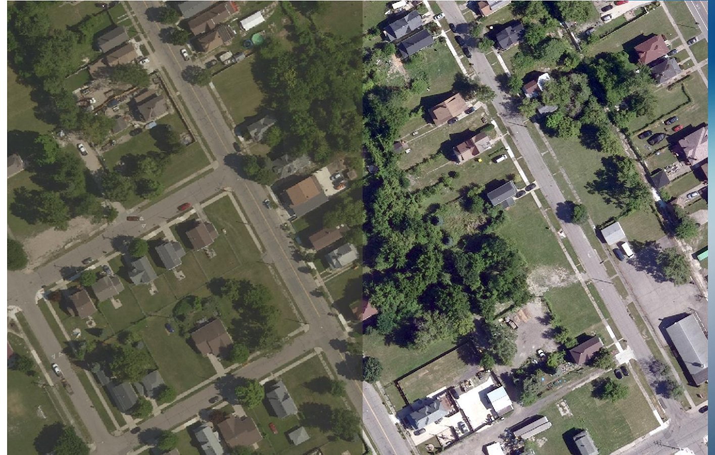
Left: Ray Traced Image, Right: Orthoimagery
